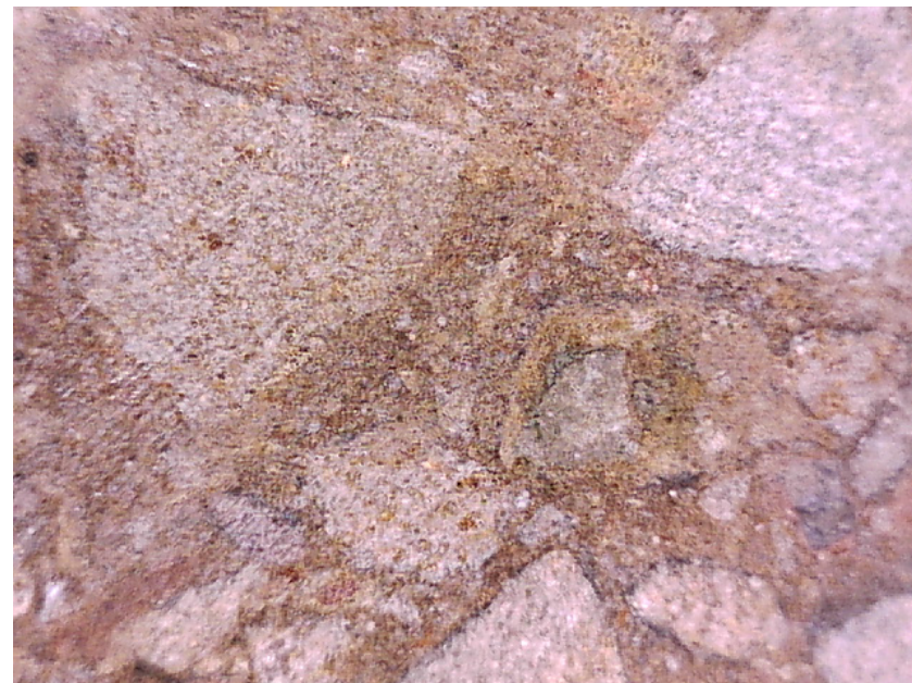
Lithic fragments (one or more minerals), quartz and feldspars (mostly orthoclase) aggregates as seen under a microscope in Brad Mimlitz's rammed earth test cylinder from the Laguna Arts Center Project.
